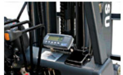
3. Connect the display to the vehicle's 12 volt power or use batteries as preferred.
